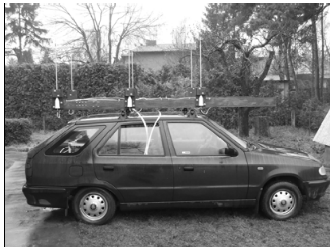
Fig. 10. Passive radar mounted on car platform
