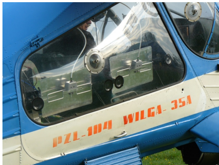
Fig. 17 Commercial DVB-T antennas used in experiment
