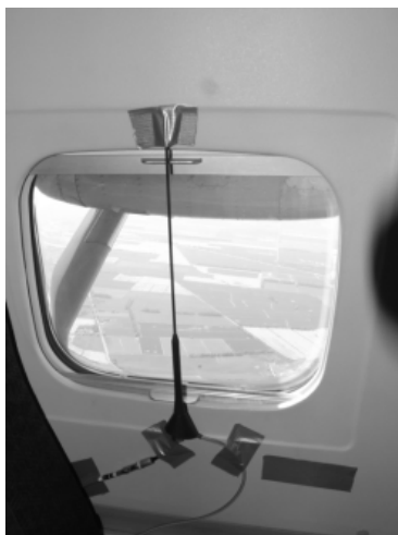
Fig. 13. PCL antenna mounted at the airplane window
